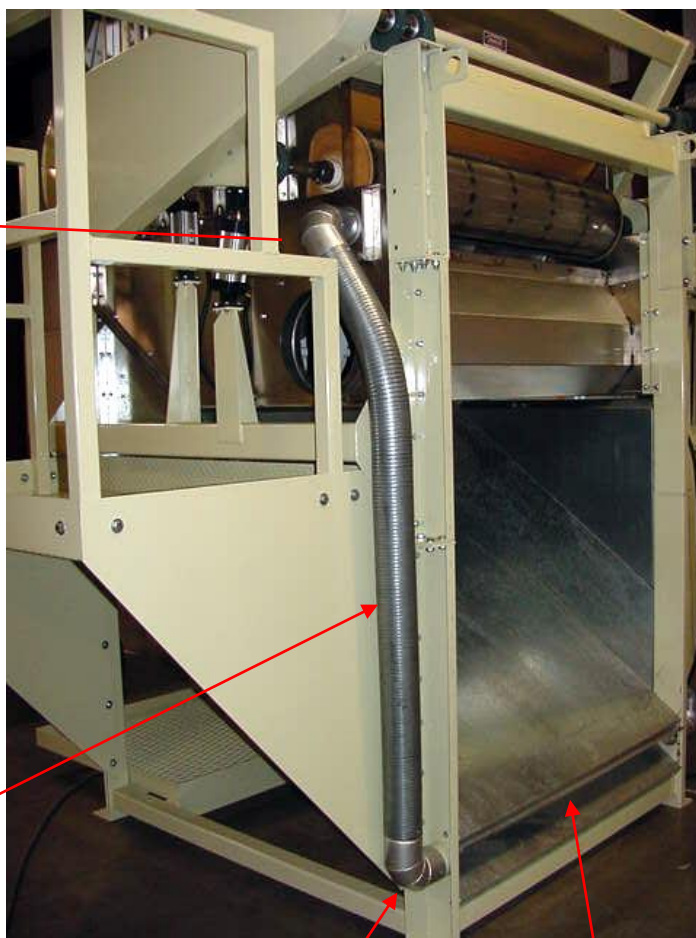
Port on each side of lower vertical support for dry hot air source with 90 degree elbow attached for hose connection.
