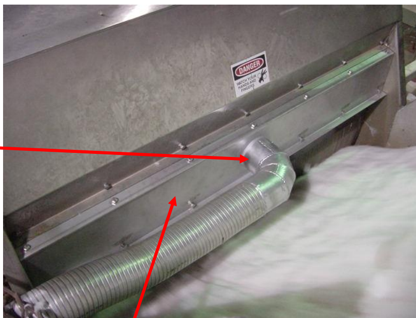
21187 SCREEN DRUM DRYER AIR BOX
