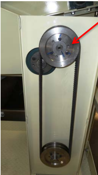
108 in-lb for SDS bushing on SPEED REDUCER and MOTOR SHEAVES
