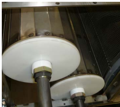
Roller housing panels shown removed allowing access to the ROLLER END WASHERS.
