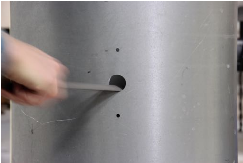
Figure 4: File the sharp edges
