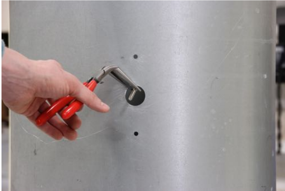
Figure 7: Install the mounting bolt with curved nose pliers
