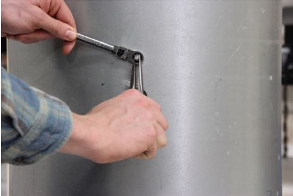
Figure 9: Tighten the lock nut while holding the bolt steady
