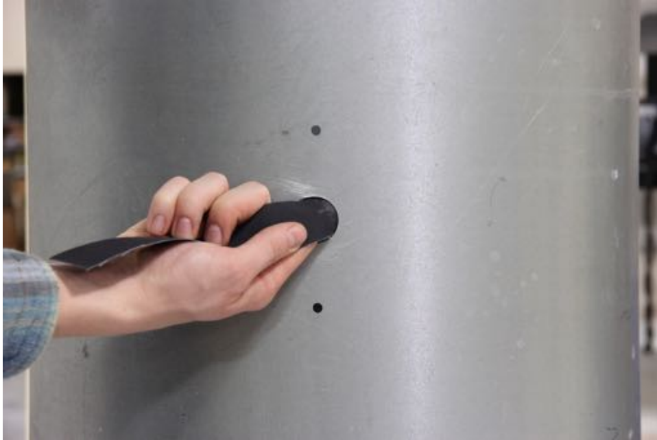
Figure 5: Sand the hole smooth
