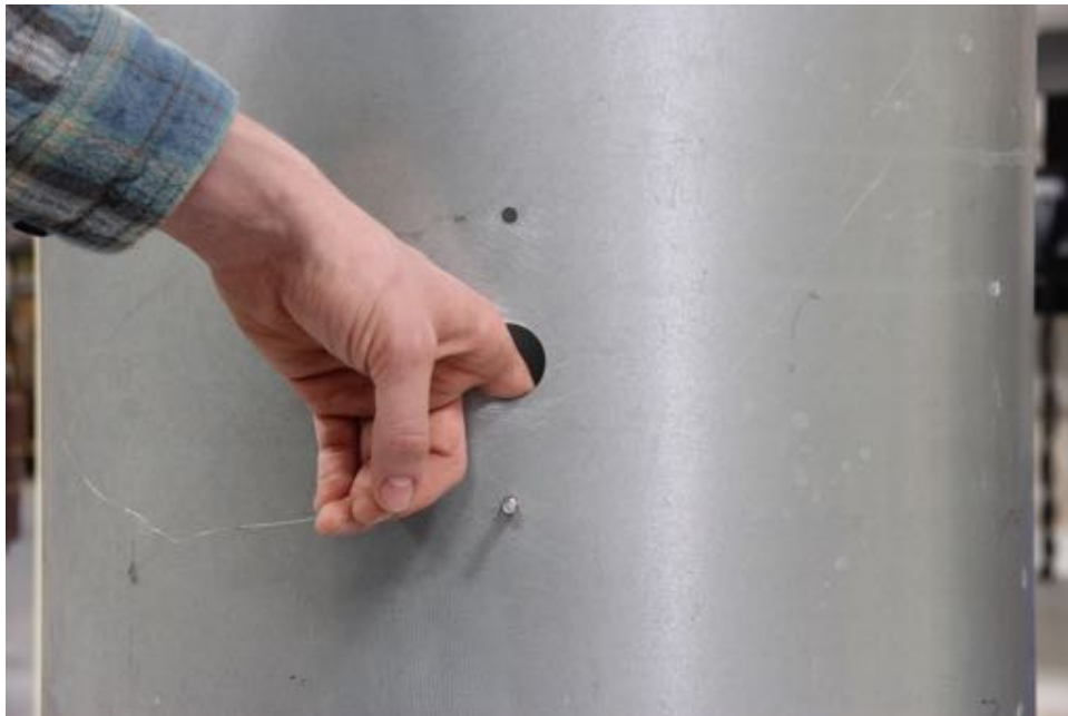
Figure 8: Hold bolt in place and thread the lock nut
