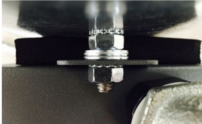
Figure: 535 detector with three washers added as a spacer.
