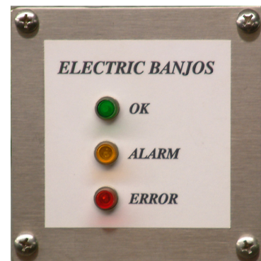
OPTIONAL 20521 BANJO STATUS PANEL (located at ginner's console) (not used with MM III+)
