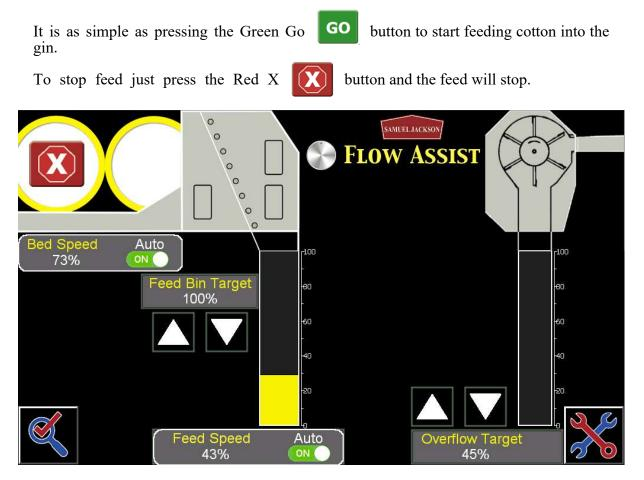
When used in collaboration with a Mirror X or Spectrum using Flow Analyzers, Flow Assist can automatically pause the Module Feeder or Feed Control when there is a Flow Analyzer alarm condition. It will also automatically begin feeding cotton again once the Alarm condition has cleared.
