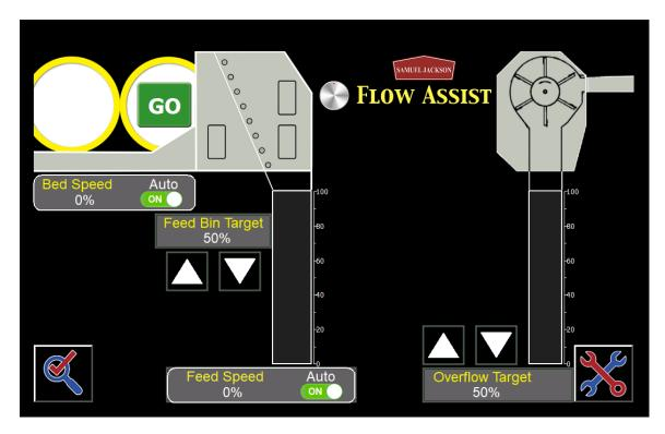
The Bed Speed can be operated in Auto or Manual.
