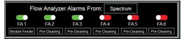
Flow Assist can pull Flow Analyzer alarms from a Mirror X or Spectrum on the network.
