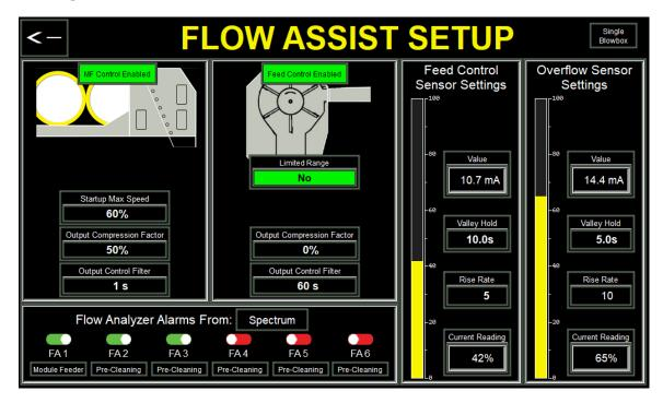
The setup screen is broken into sections, Module Feeder, Feed Control, Feed Control Sensor, Overflow Sensor, Flow Analyzers.
