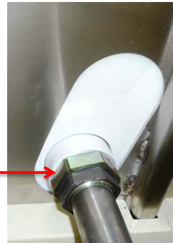
3300 in-lb for KEYLESS BUSHING
